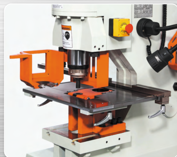
*雙孔下模座可沖50mm以下尺寸(為S/SD/KD及PM機型標準配件)
